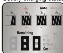
Battery Temperature Warning
